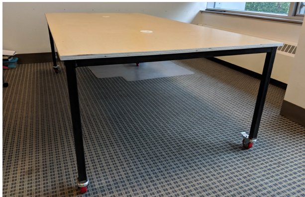
4' x 8' desk for Olin Provost - maple plywood, welded steel frame, inset power, locking casters
